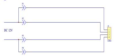
(3) Main power supply & charging capacitor wiring diagram
